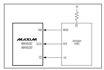
Figure 4. SPI/QSPI Interface Connections
