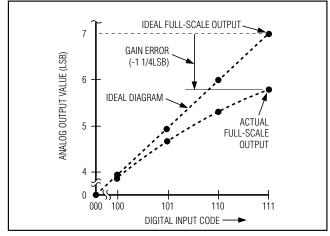
Figure 6d. Gain Error
