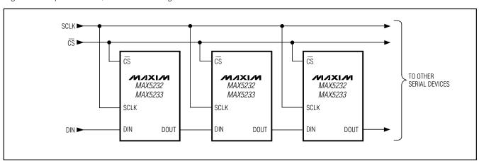
Figure 10. Daisy-Chaining MAX5232/MAX5233 Devices
