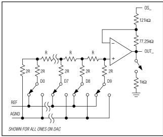
Figure 3. Simplified DAC Circuit Diagram
