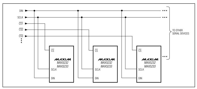
Figure 9. Multiple MAX5232/MAX5233s Sharing a Common DIN Line
