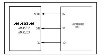
Figure 5. Connections for MICROWIRE
