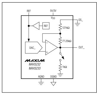
Figure 7. Unipolar Output Circuit (Rail-to-Rail)
