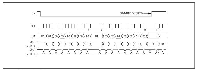
Figure 1. Serial Interface Timing
