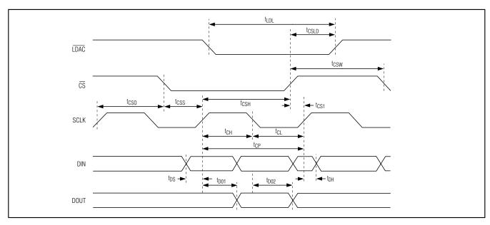
Figure 2. Detailed Serial Interface Timing
